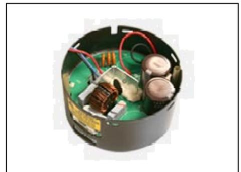
So what can be programmed into the ECM 2.3 motor? Options include a variety of characteristics, including the rotation direction of the motor, start and stop ramp rates, on and off blower delays, speed (i.e. - rate of rotational motion) of the motor and torque (i.e. - rotational force or power output down a shaft) of the motor. Unlike conventional PSC motors, which are designed to operate at one speed, ECM 2.3 variable-speed motors can run over a wide range of speeds. This
